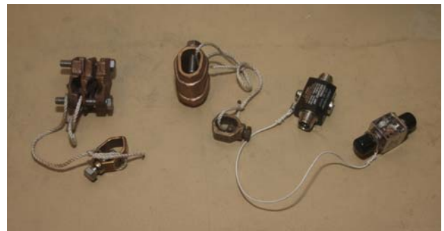
Stan circulated several types of grounding clamps and in-line lightning protection devices.
