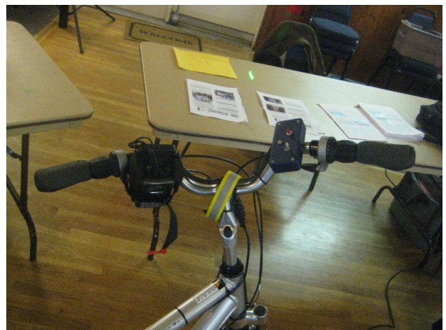
Dick W1LTN showed his set up for bicycle mobile with the rig on the left, the key switch on the right, and the antenna mounted on the back which you cannot see.
