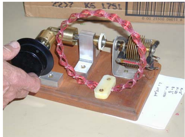
Show and Tell from Earls machine shop above and below a right angle drive called a "Hookes right angle coupler" used to drive a tuned circuit using a basket weave coil.
