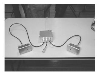
San KD1LE showed a portable mast system and fold up two meter ground plane antenna he made for portable as well as emergency use.
