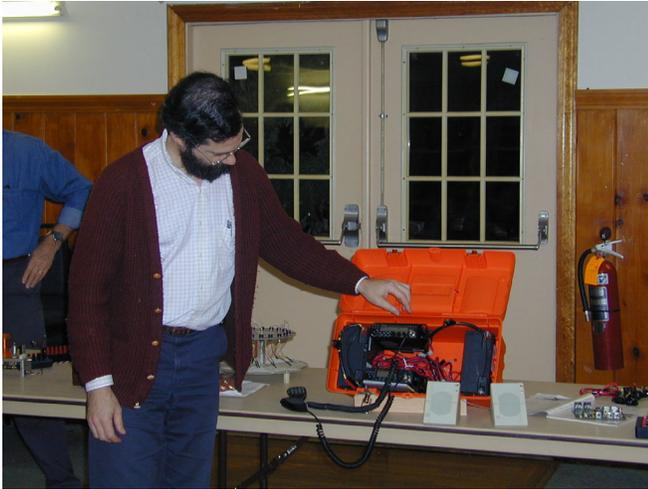
Ralph KD1SM, ARES box with two mobile rigs and batteries for rapid deployment, Powerpole distribution box with recessed connectors and individual circuit fuses
