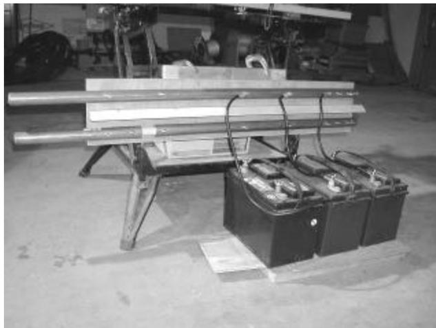
To put real numbers on the battery conditions Bob W1XP built a load that could simulate the combined three transmitter current draw of 35 amps. We then tested each battery under load for an extended period and then recharged them.
